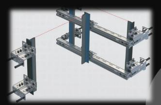
All bracket are 5mm HR material, **Pre-treatment** seven tank and Micron minimum 25 process PHOSPATING coating **Powder** minimum thickness 60-80 Micron
